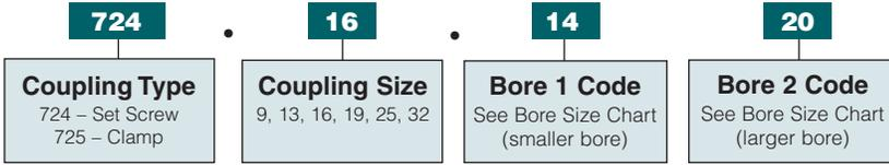
Order as one complete coupling part number with two bores. Include (.) in Part Number.
