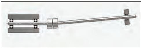
**Fig. 6** A semi-floating shaft located by a self-aligning bearing at one end should be supported with a single-stage coupling at the other.
